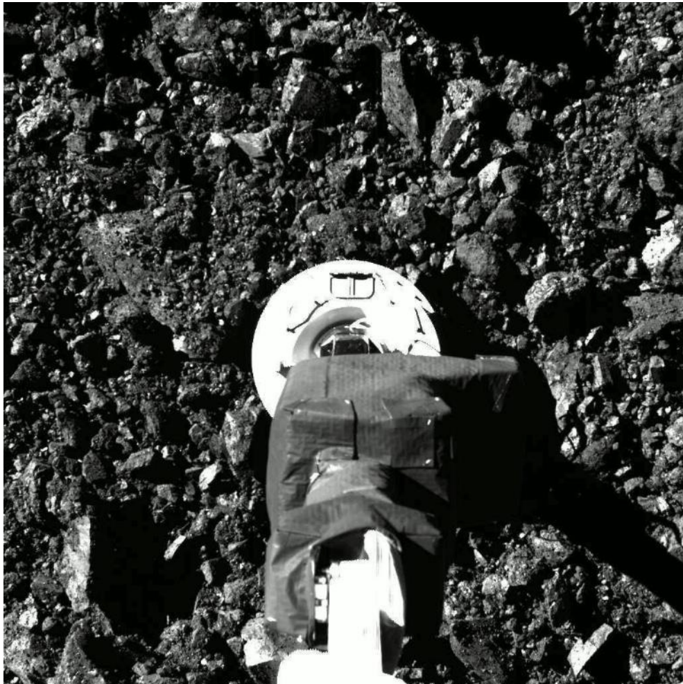
FIGURE 2.22 OSIRIS-REx sampling the asteroid Bennu on October 20, 2020. The sampling head is one-foot wide. SOURCE: NASA/OSIRIS-REx.
