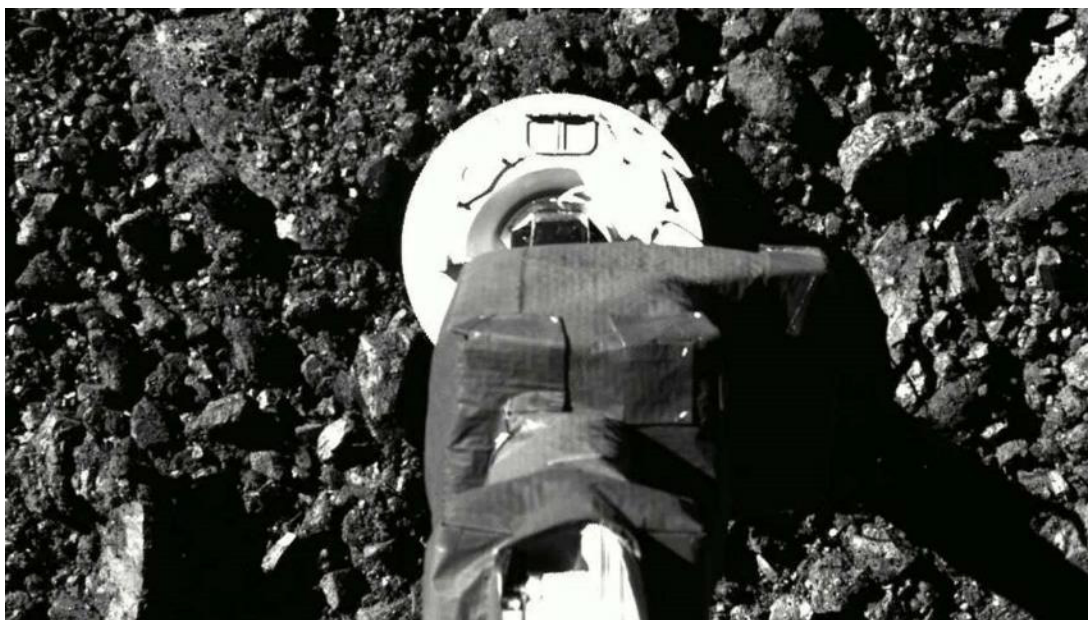
FIGURE 1.6 OSIRIS-REx's sampling arm in the process of collecting material from the surface of the asteroid 101955 Bennu in 2020. SOURCE: NASA.
